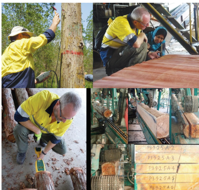
Figure 4. The BFC E. pellita wood quality programme showing measurement of Acoustic Velocity in at four-year-old tree (1), veneer sheet with good qualities for both appearance and industrial ply (2) and detailed assessment of sawn boards (3).
