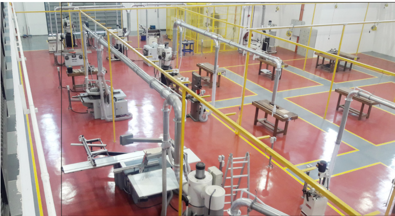
Woodworking machinery with full system of integrated automatic dust collection.
